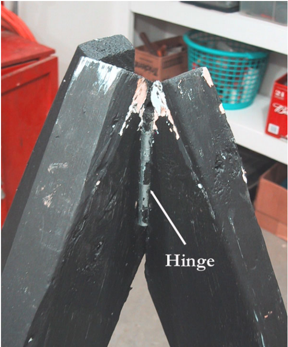
Photo 4. Detailed view of the top of the tripod from the opposite side, showing the hinge placement.
