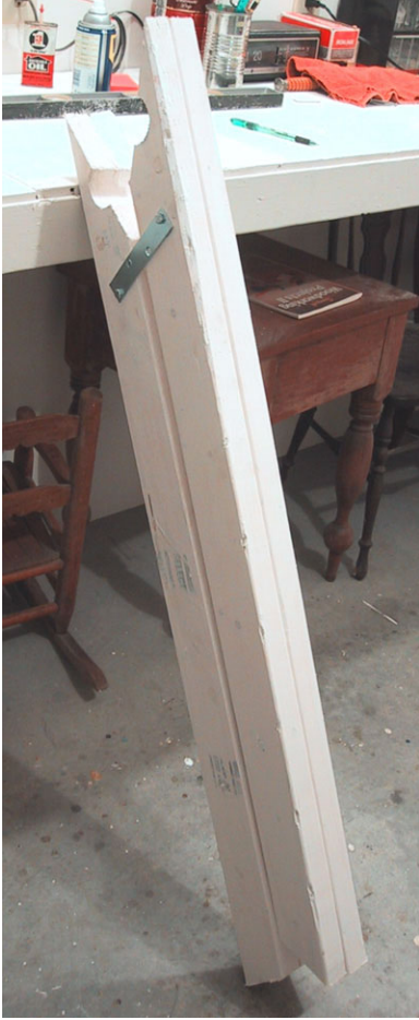
Photo 11. "A" brace in folded position for transport and storage.
