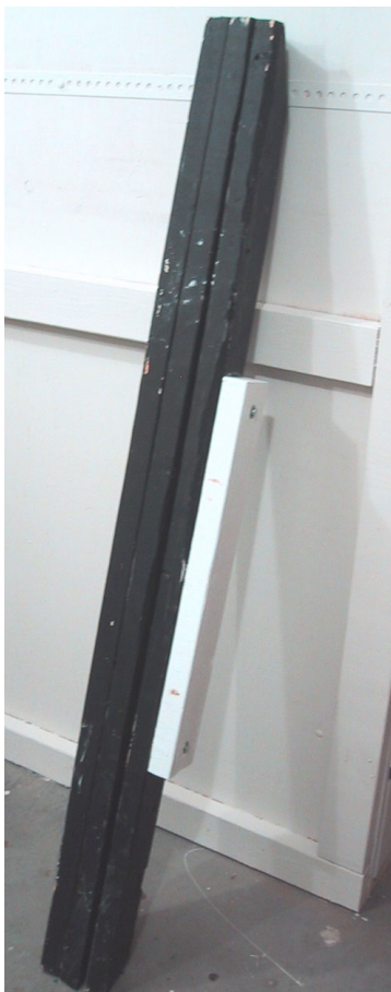
Photo 6. Tripod fully folded for transport and storage.
