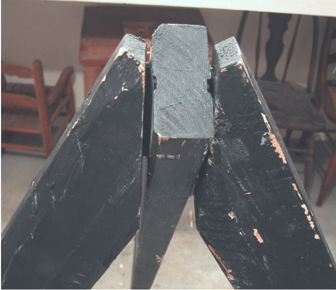
Photo 2. Detail of top of tripod. Legs fold away from this side.
