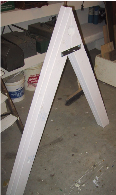
Photo 8. A brace set up in the position that would hold up the middle of a bike rack. The conduit fits through the 2.125" hole near the top of the "A." Notice that the 2x4 legs are doubled for strength. For example, a four-section bike rack filled to capacity with bicycles would be a nearly 1,500 pound load.
